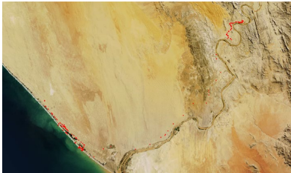
Data mapping showing the remote operating geography of the customer mine and location of drowsiness warning events (red dots) transmitted from Optalert systems via radio network
