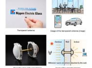
shape of the lens, radio waves can be transmitted in a certain direction or over a wide range. The lens is not subject to deterioration caused by ultraviolet rays because it is made of glass. It can be used stably over a long period in various places, both indoors and outdoors. neg.co.jp
